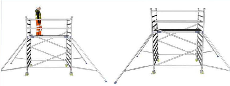
1.26 Stand on the platform and ensure the guardrail are securely in place, at the opposite end of the tower.
