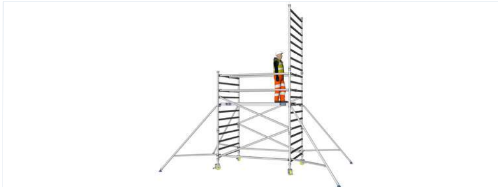
1.26 Stand on the platform and ensure the guardrail are securely in place, at the opposite end of the tower.
