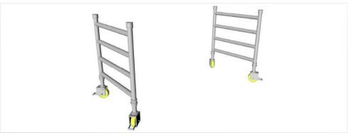
1.5 Clip the horizontal brace onto the frame. Connect the brace directly above the casting at the first horizontal rung position.
