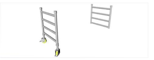
1.4 Insert the adjustable leg, then the castor into the bottom of the frame.
