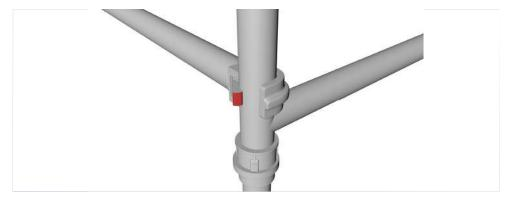
1.8 Insert the next section – this may vary in size depending on which tower you have. However, the image we have used, is an 8 Rung (2m high) frame.
