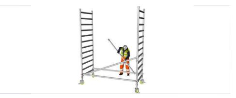
**1.11** Clip the diagonal braces onto the lowest rungs.
