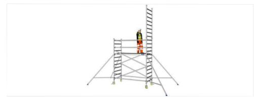
**1.26** Stand on platform and ensure the guardrails are securely in place at the opposite end of the tower.
