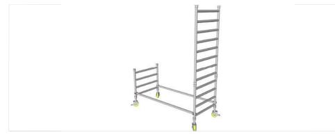
1.9 Clip the diagonal braces onto the lowest rungs.
