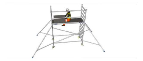
**1.22** Ensure at this point the diagonals are also in place.
