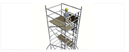
1.43 Stand on platform and ensure that guardrails are securely in place at the opposite ends of the tower.
