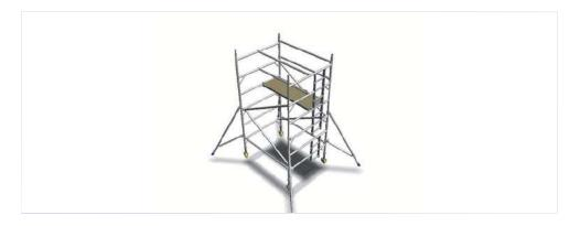
**1.28** Stand on platform and ensure the guardrails are securely in place at the opposite end of the tower.
