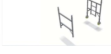
1.4 Insert a leg and castor assembly into the bottom end of a span frame.
