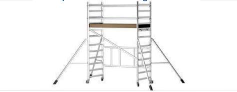
Add additional frames by climbing through the hatch then place 1.17 hatch deck at required platform height. Secure hatch platform with locking braces, repeat steps 1.11,1.12, 1.13 & 1.15
